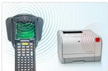
RFID technology (radio frequency identification) allows you to use radio waves to identify objects of property automatically. To do this, to the objects (in our case - tables, chairs, computers) special programmable RFID tags that are recognized by RFID-reader from a distance of 5-8 meters are attached. The information read from the tags is sent to the accounting system and can be checked at any time.
